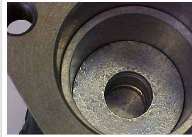
Figure 28 – Ten Spacers Installed in Piston.
