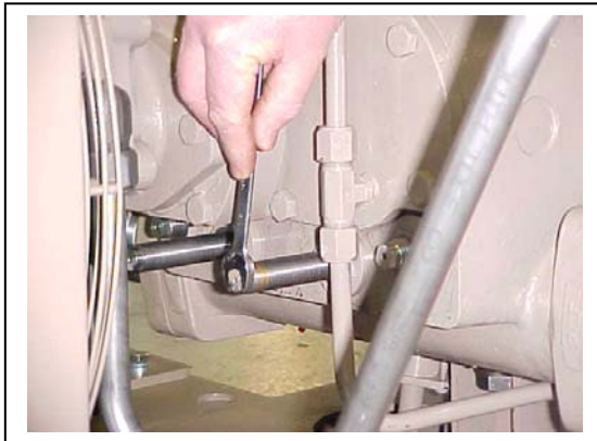
Figure 10: For MEDIUM Vi, turn the inner valves counterclockwise until they are fully out.
