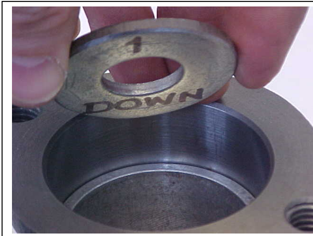
Figure 26 - Installation of First Spacer. Marked "1". Install "Down" side down (chamfered to keep sharp edges from I.D. of piston)
