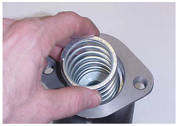
Figure 29 – Installation of Spring Part No. 24-810. Either end may be installed down.
