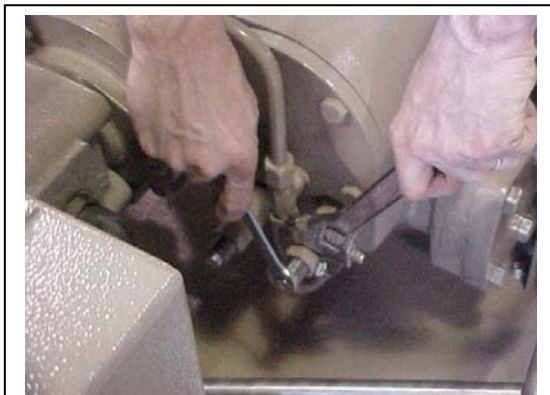
Figure 12: Reinstall and tighten locknuts just snugly while holding valves so they do not turn. The valve positions in this figure are low Vi. Note that all of the valves are out. PERIODICALLY LUBRICATE THE VALVE STEM THREADS WITH GREASE TO PREVENT RUST AND ALLOW FOR FUTURE ADJUSTMENT.
