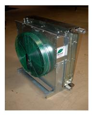
These units are three feet wide by three feet tall by twenty inches deep with a 30" fan that can blow in either direction. They are designed with an oil section that can cool a screw compressor ranging from 40 to 200 horsepower.
