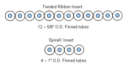
This illustration shows that for lube oil cooling services in air coolers, four (4) 1" SpiralX finned tubes will transfer the same amount of heat as twelve (12) 5/8" finned tubes with twisted ribbons.
